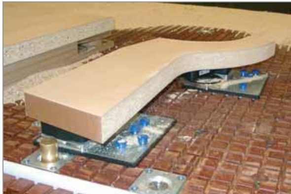
Innospann vacuum blocks for grid tables, freely positionable on the Mini-Plate ISMP-R
